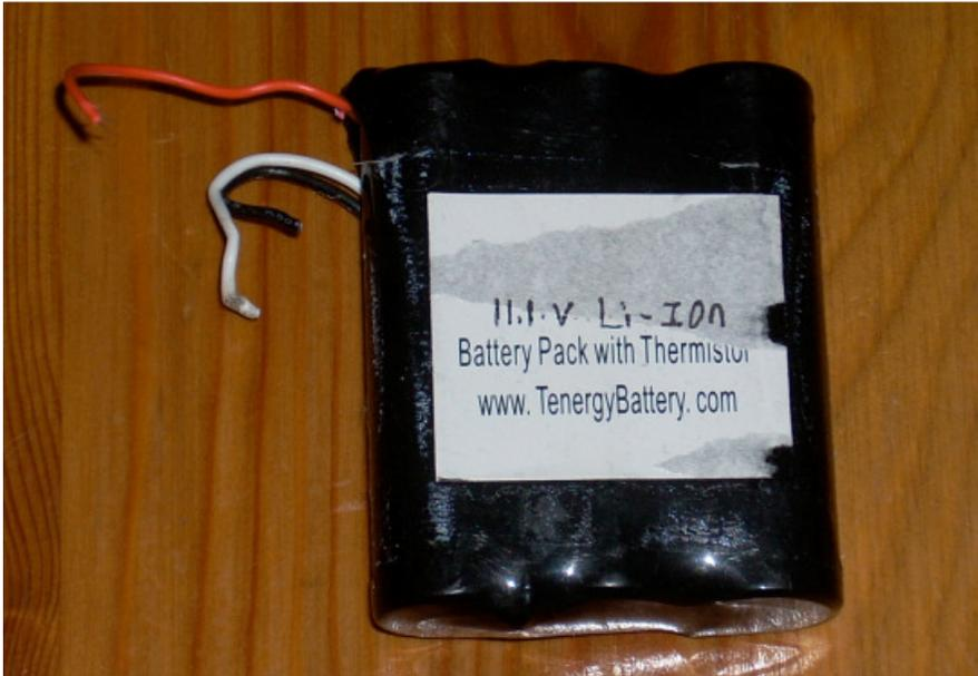
Figure 6: Standard battery used in VAST. Red is positive, black is negative, and weight is thermistor.
