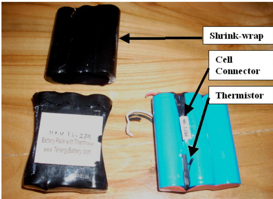
Figure 7: Two shrink-wraps enclose the three cells. This battery back is identified with the manufactures name (Tenergy). The cells are 18mm in diameter and 65mm long, which puts them in the 18650 size class. A web search for *Tenergy 18650* would be enough information to find the specific datasheet for these cells. Note, the Cell Connector provides an electrical connection and is included for manufacturing purposes only. It does not serve any other purpose.
