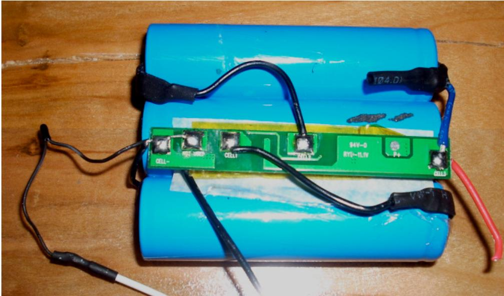
Figure 8: This balancing circuit keeps the individual cell voltages the same and is the reason external balancing mode is selected when charging these batteries. Some lithium ion batteries come with a built in thermistor to sense battery temperature. A thermistor is a type of resistor whose resistance varies detectably with temperature. If battery temperature is not an issue the white wire can be disregarded/cut.
